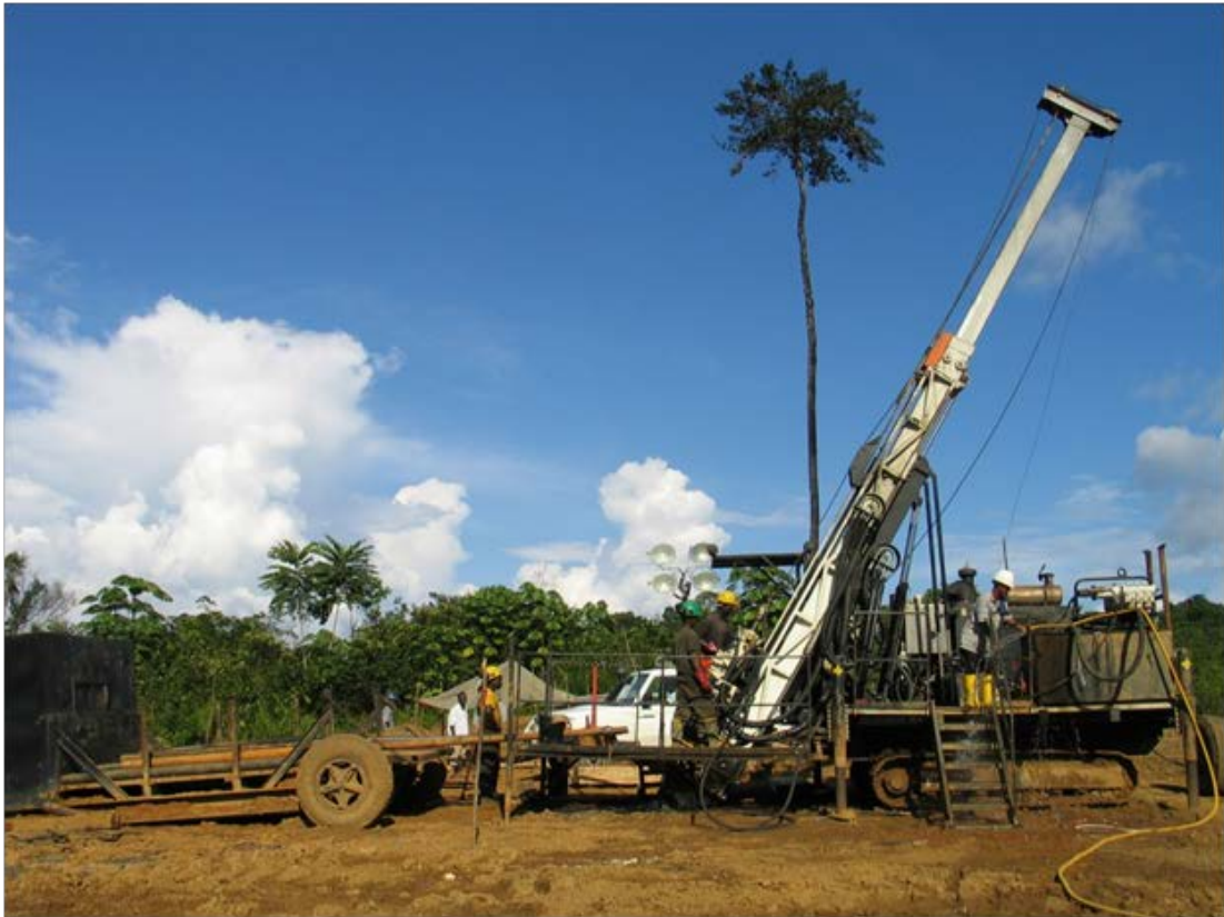
Figure 10-3: Diamond Core Drill Rig
